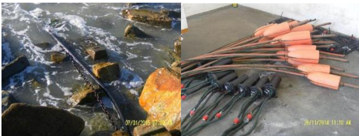
Figure E1 Shark Repellent Cable. Left: cable leaving shoreline, Right: cable floats and controls. Source: Jeremy Cliff.
