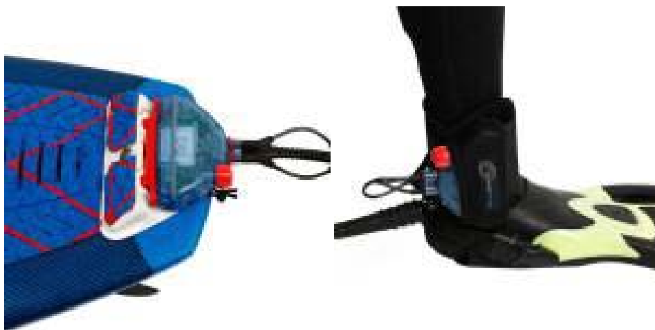
Figure F1 Shark Shield devices. Left: surfboard device fitted to rear of the board. Right: attached around the leg of a snorkeler. Source: Lindsay Lyon.
